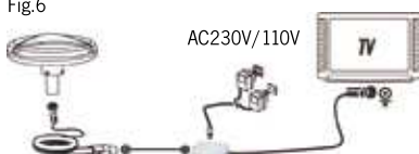
Installation 1: Directly connected to TV(Fig.6)
